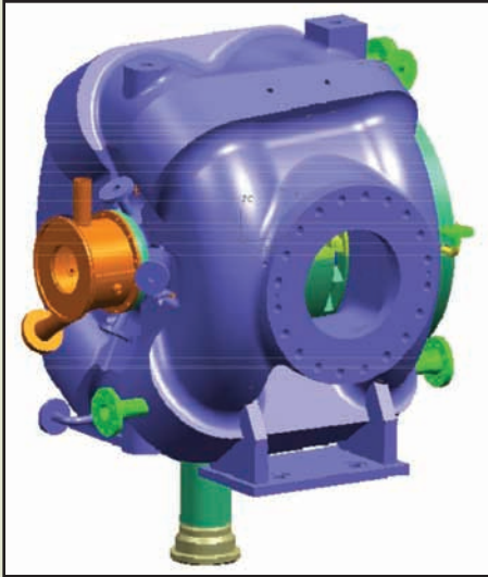
Figure 4. Compressor casing. Bearing span 35 inches.
