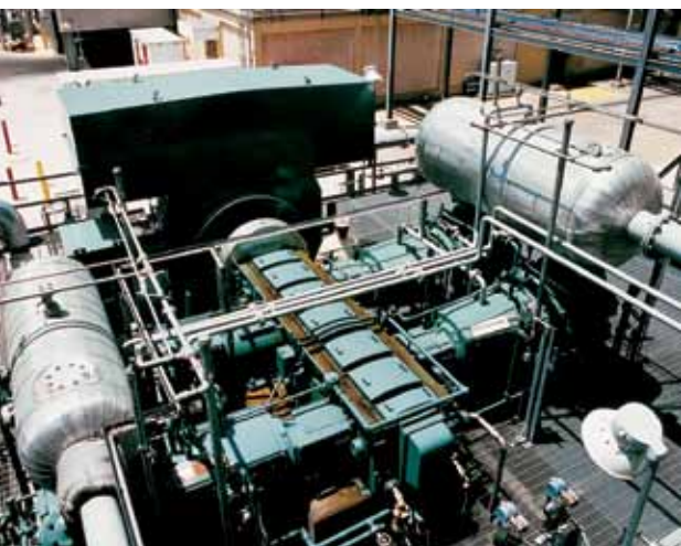
Foundation-mounted HHE-VB unit with spread center frame that provides additional maintenance access between cylinders. Note manifolded suction pulsation vessels with banded insulation.
