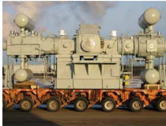
In February 2005, Dresser-Rand provided APCI with two skid-mounted, HHE-VL compressors, each including a frame lube oil console attached to the skid.
