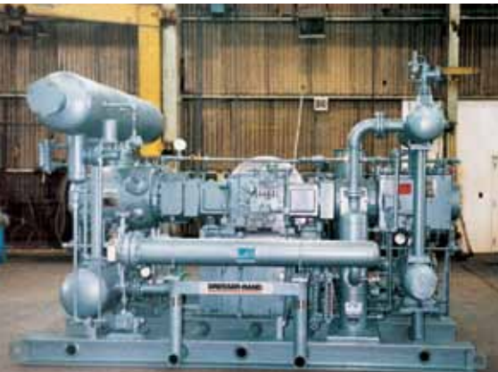
Skid-mounted, 125 hp, two-cylinder PHE package being prepared for shipment. Depending on the physical size of the compressor, skid mounting saves field assembly time.
