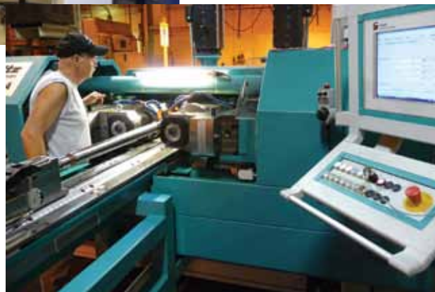
The quality of rolled threads can lead to major field problems. Our new digitally controlled thread rolling machine is used in the manufacture of all piston rods.
