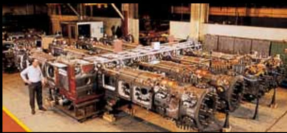
12,000 hp, eight-cylinder HHE-VL in our factory assembly area being prepared for barover and rod runout alignment checks.
