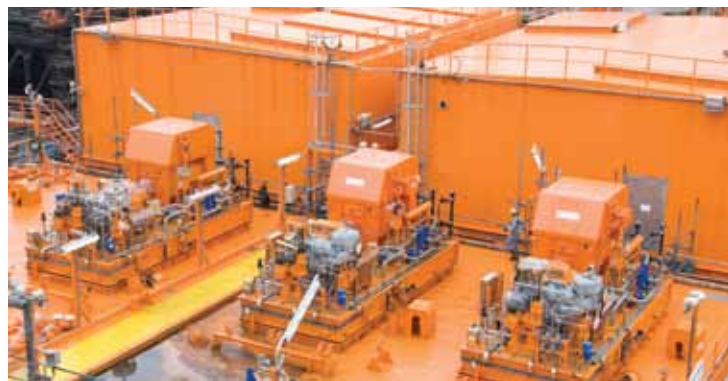
Three 5 MW steam turbines supplied to Aker Floating Production.
