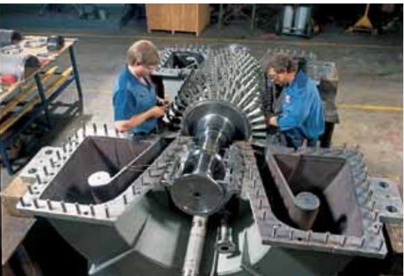
Installing axial air compressor rotor into compressor housing.
